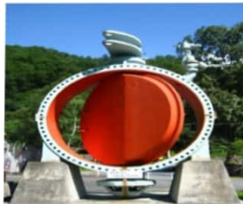
Fig: Valve used to ON/OFF water flow
